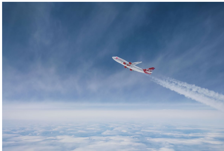
Cosmic Girl pitches up at a sharp pitch angle to simulate the release maneuver during a cryogenic captive carry flight. April 2020.
